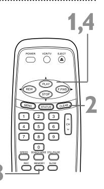
To go to a tape location where the counter was reset to zero, press REW or F.FWD when play is stopped. When the tape reaches zero, it will stop. Press PLAY to watch the tape.
